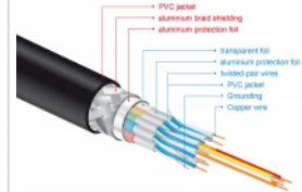
Triple shielding for lossless signal transfer
